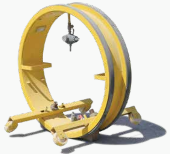
Fig 18 Testing device for the single joints
