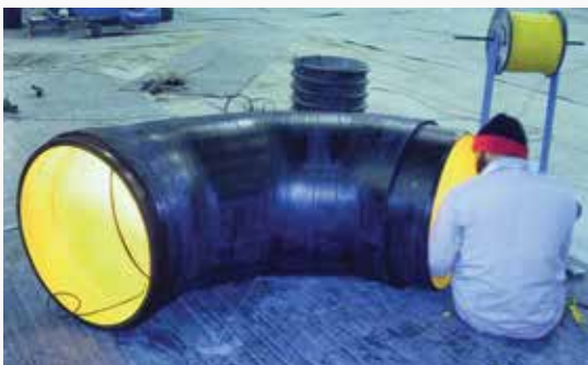
Bend for NIC HDPE Corrugated Pipe, with socket and spigot, for project in Iraq
