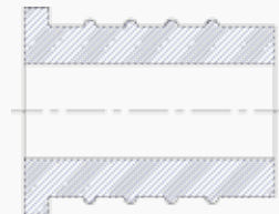
Rubber Plug to hold cable in HDPE subduct.
