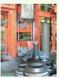
The company's concrete pipes factory is the largest and most modern of its type in the Middle East, with a yearly production capacity of 250 km (linear). Due to the modern technologies owned by NIC and its integrated quality control program, this factory is a leader in its field. Pipes are produced by mixing the semi-dry concrete mixes by means of the vertical casting method using the latest procedures in the field of vibration technology.
