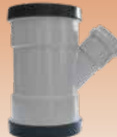
Reduced Junction 45° (Y) Rubber Socket 110x50, 110x75mm
